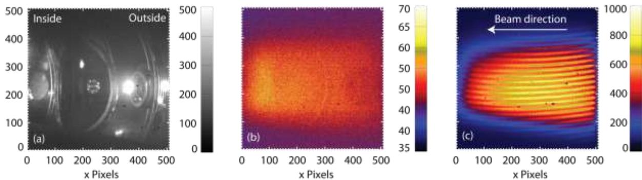
Figure 17: Left: The camera view of the internally illuminated TEXTOR vacuum vessel. Centre: continuum plasma emission near 662nm (no beam) and Right: The image when the neutral beam is activated. Visible interference fringes indicate that the light is polarized. The phase of the carrier fringes conveys the polarization angle of the MSE multiplet from which can be deduced the internal current distribution.
