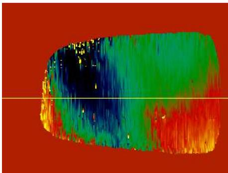
Figure 18: Typical demodulated polarization tilt angle image. The observed spatial variation in pitch angle conforms well to expectations based on simple models of the internal current distribution.
