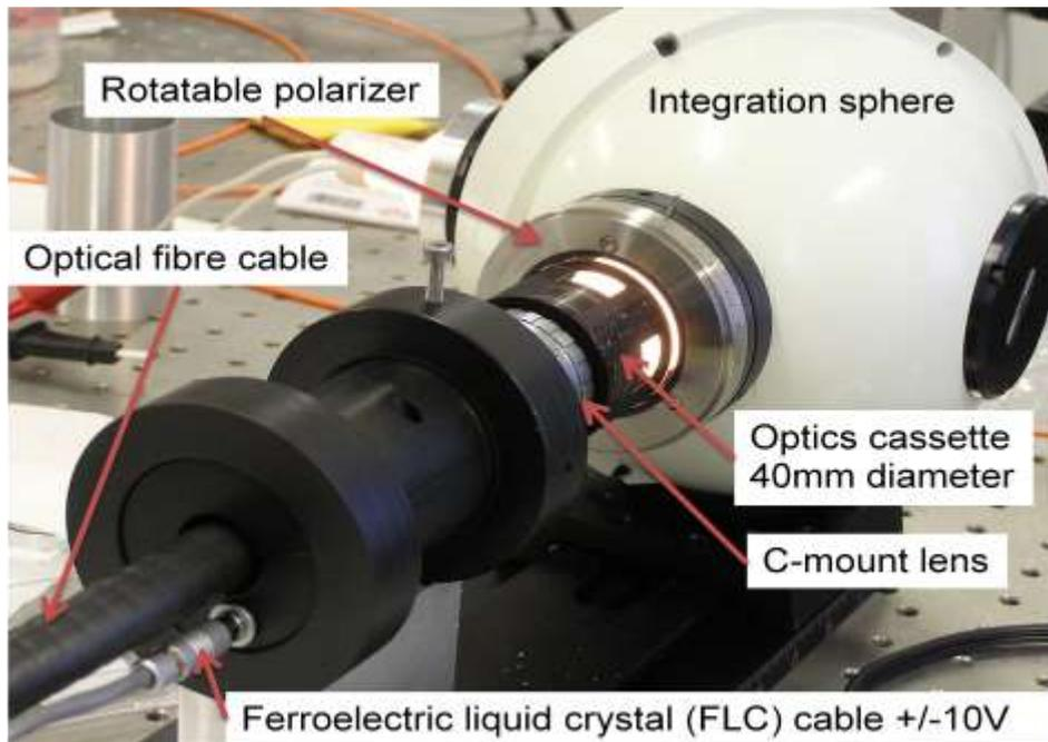
*Figure 15: Photograph of the front-end optical cassette, c-mount lens and optical fibre cable installed for first internal current imaging experiments on the TEXTOR tokamak in Germany. The back end of the imaging optical fibre bundle is imaged by a fast CCD camera. In this photograph, the system is being calibrated using diffuse light from an integrating sphere.*
