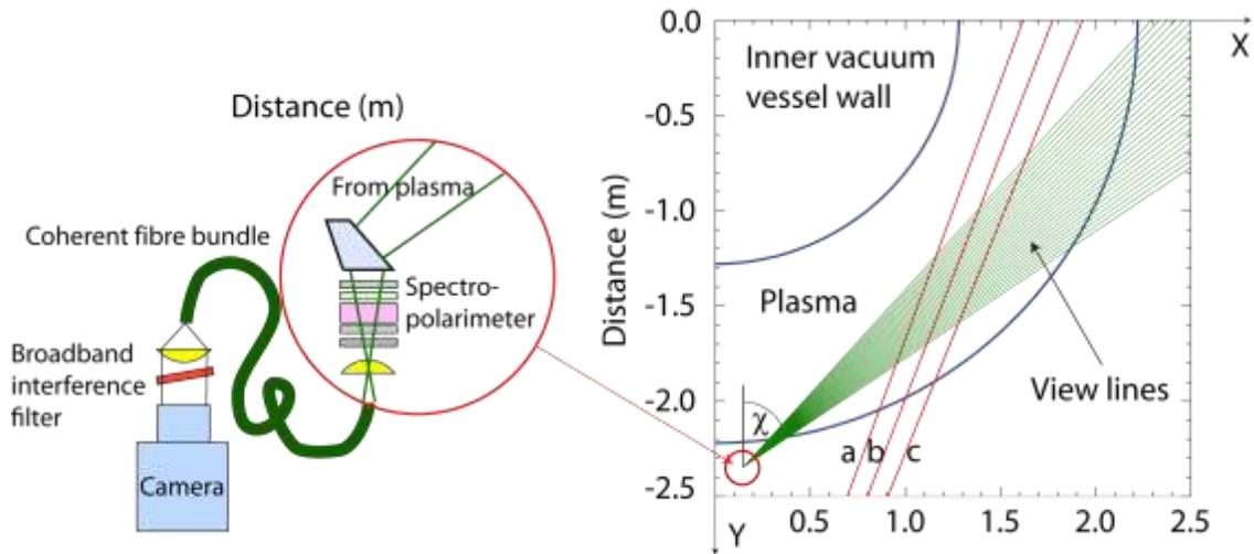
Figure 16: The TEXTOR system geometry. The neutral beam spans the region designated by the lines labelled 'a', 'b' and 'c'. The green lines represent the span of the camera lines of span. A coherent fibre bundle transports the image to a broadband interference filter and CCD camera.
