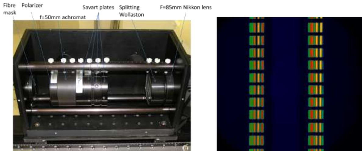
*Figure 19: Left: Photograph of the imaging interferometer shipped to JAEA. Right: calibration images of white light source fringes for a vertical array of input optical fibre channels. Left and right hand image pairs are in antiphase.*
